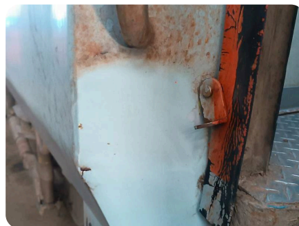
Coach body corner. Grime lifted off, paint intact.
